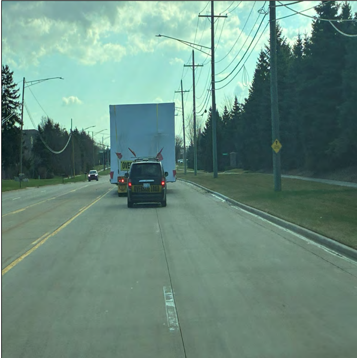
Figure 8 – Transporting 2MW E-House @ Eastbound 15 Mile
