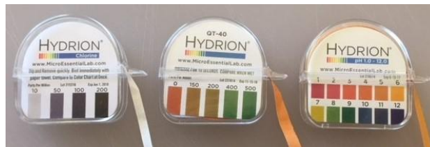
Test strips for chlorine, quat, and acid sanitizers
