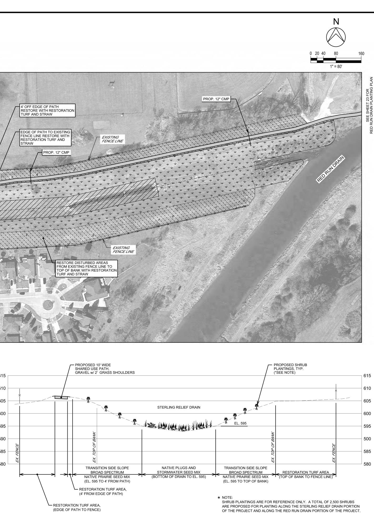
TYPICAL SECTION THROUGH STERLING RELIEF DRAIN (LOOKING EAST) SCALE: 1" = 20' HORIZ. 1" = 10' VERT.
