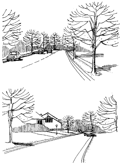
Illustration 4.16. Implement road standards such as narrower widths, sidewalks on only one side, and roadside swales to minimize impervious surfaces and encourage infiltration.
