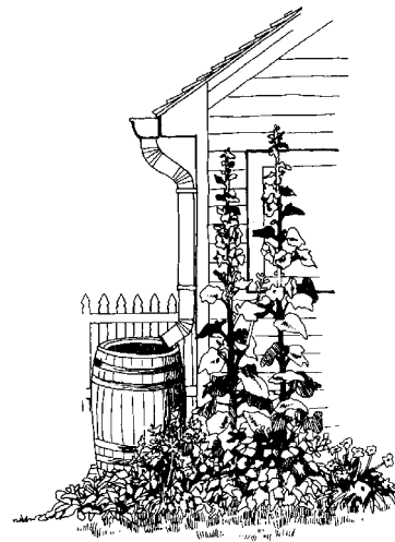
Illustrations 4.12. & 4.13. Limit storm water runoff using rain gardens and rain barrels.
