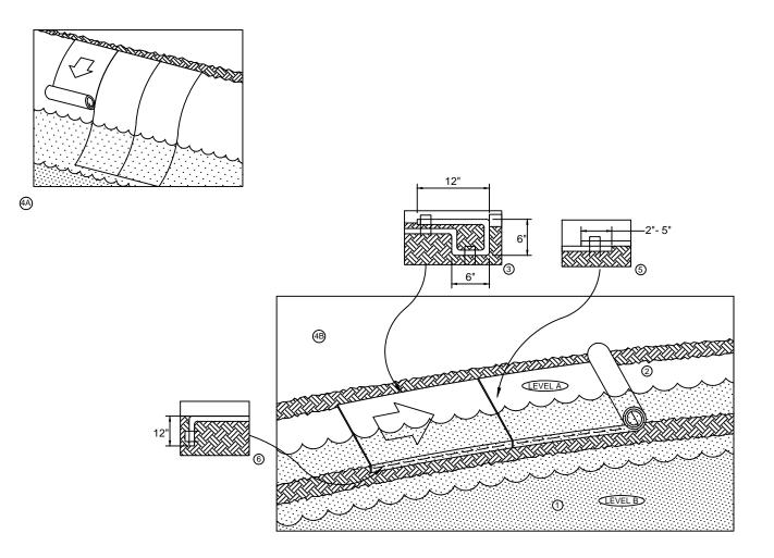
1. FOR EASIER INSTALLATION, LOWER WATER FROM LEVEL A TO LEVEL B BEFORE INSTALLATION.
