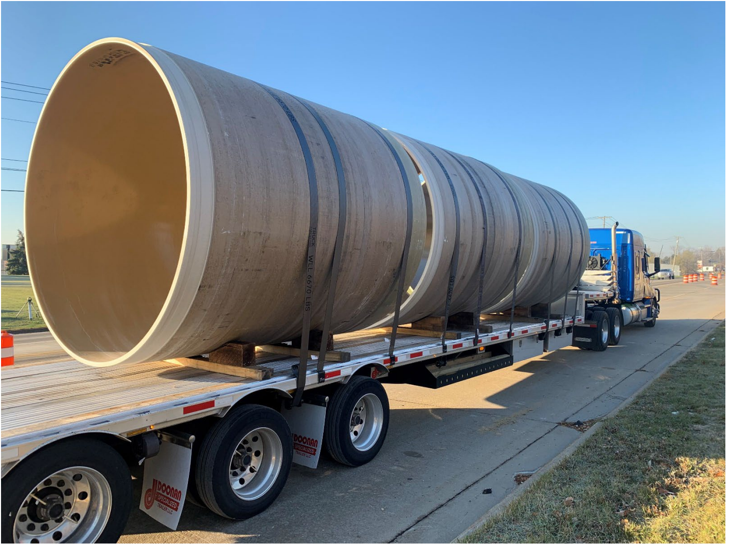
Figure 9 – 9' 2" Diameter HOBAS Delivery – Romeo Arm Curve Lining
