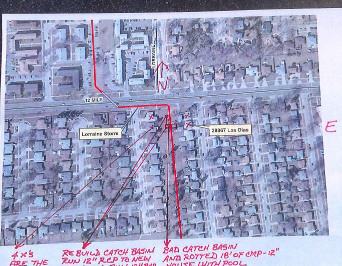
AXS REBUILD CATCH BASING ARE THE RUN 12" RCP TO NEW 4 HOMEOWIE CB NORTH-RUN 12" RCP REAR YARDS EAST TO TAP 11" PIPE
