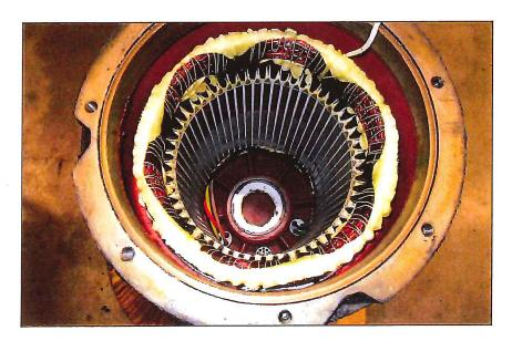
• The stator is dry and passes all electrical testing
