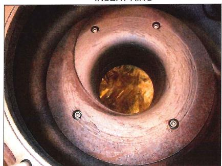
The insert ring has minor wear and will be reused
