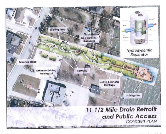
**Need:** A recently completed stormwater asset management study found that while the 11.5 Mile Relief drainage system was in good structural condition, sediments and trash were being transported through the pipes directly into Lake St. Clair. Due to over 50% imperviousness and lack of stormwater treatment in this highly urbanized watershed, areas where green stormwater infrastructure can be implemented to reduce stormwater pollution into the lake are limited.
