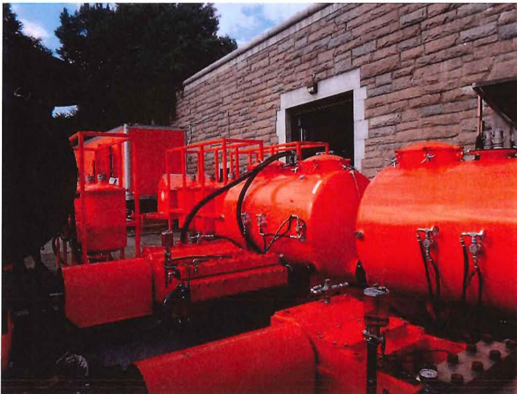
High pressure pump unit.
